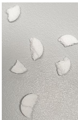
Figure 73: MPT: Capa (40:60%, w/w) tablet manufactured by DC technology
