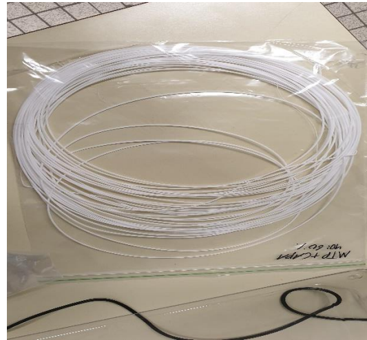
One of the printed filaments (MPT: Capa 40:60%, w/w)
