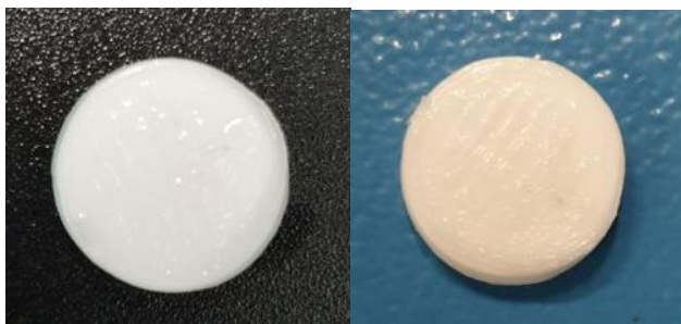
Figure 62: MPT: Capa (40:60%, w/w), before and after dissolution
